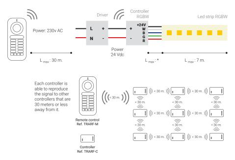
\*Maximum length of 2 metres for a wire with length section below 0.5 sq.mm. For more than 2 metres, use a wire of 1.5 sq.mm. section.
